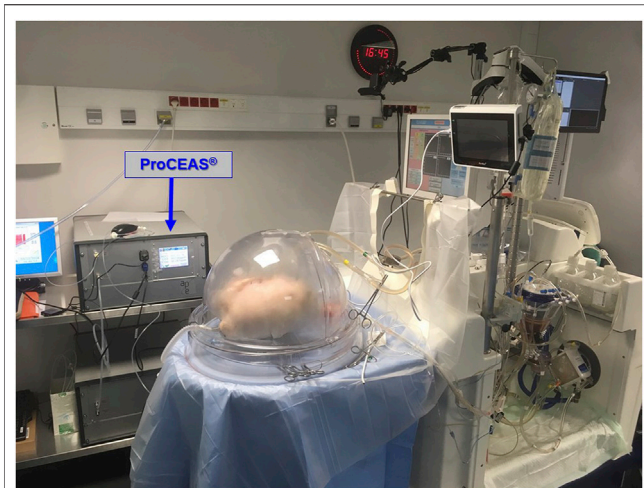
FIGURE 1 | Overview of the setup of EVLP preparation with the XPS™ device on the right and the ProCEAS® in the background, monitoring eCO in real-time. In the front plane is the ventilated and perfused ex-vivo lung.
