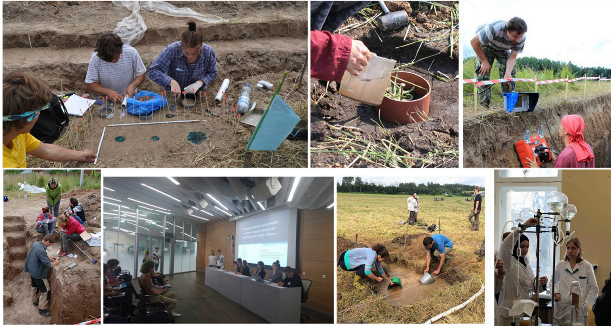
FIGURE 6 | A comprehensive set of field and laboratory activities during soil science training in Chashnikovo and MSU: From left to right: (1) an experiment using Brilliant Blue dye to trace preferential water flow paths in soil profiles; (2) pressure filtration rate measurements across soil horizons; (3) evaluation of soil gas emissions; (4) morphological description of soil profile; (5) a student-led conference presenting results from hands-on soil physics practice; (6) flooded soil profile inspection after rainfall; and (7) filtration experiments.
